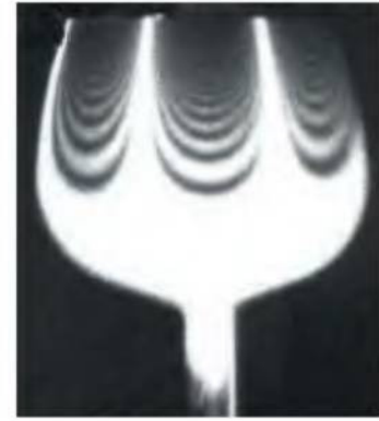
An optical technique called interferometry reveals the bell-like vibrations of a wine glass.
